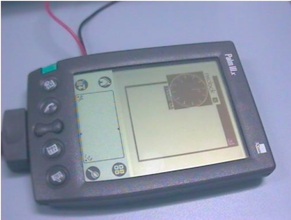
Figure 3. uClinux Running on a Real Palm IIIx (with Microwindows)
