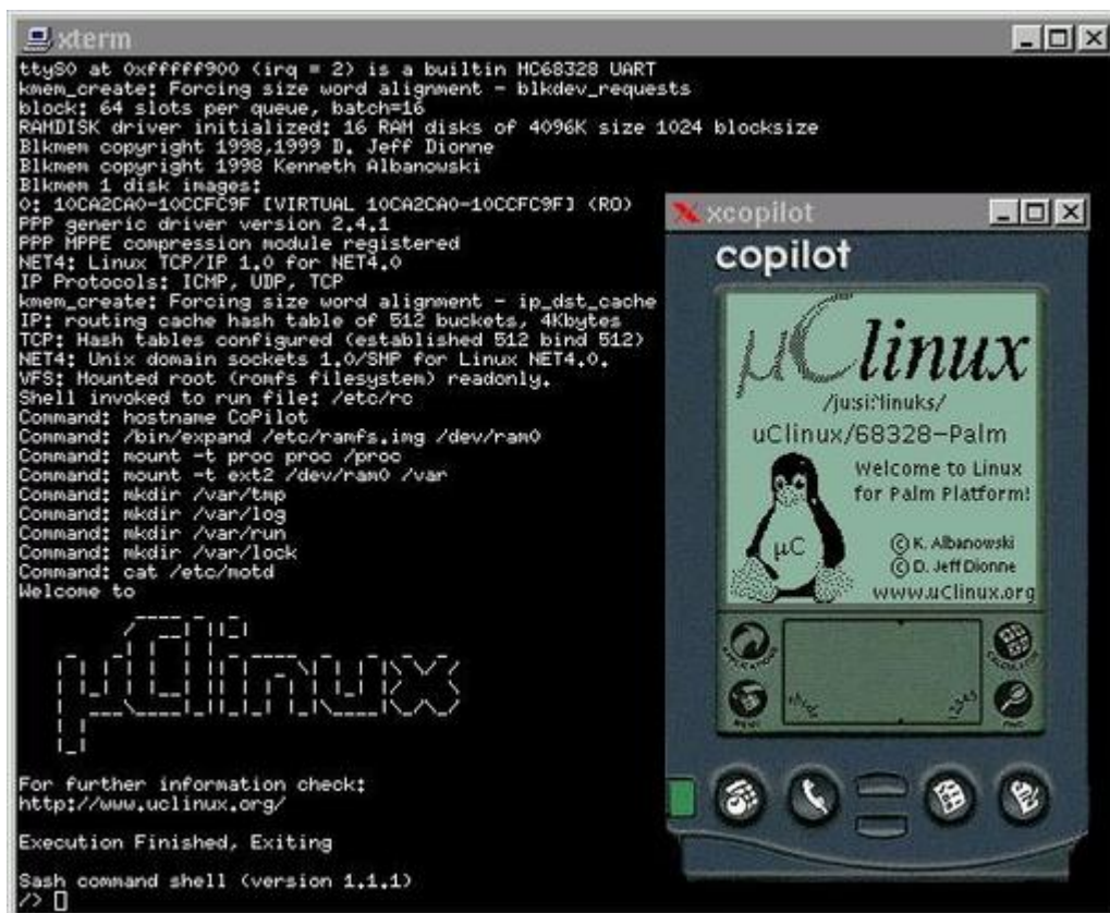
Figure 2. uClinux Running under Xcopilot (Palm Emulator)
